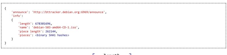
Note: pieces here would be a 51 KiB value ( $\begin{bmatrix} length \\ piece length \end{bmatrix} \times 160 = 414080$  bits).
